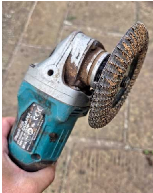
The tool for the job: a cordless angle grinder with a wood carving disc.
